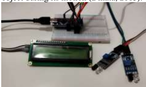
Figure 2. Arduino Nano Connected to the Breadboard, LCD Screen, and IR Obstacle Sensor
